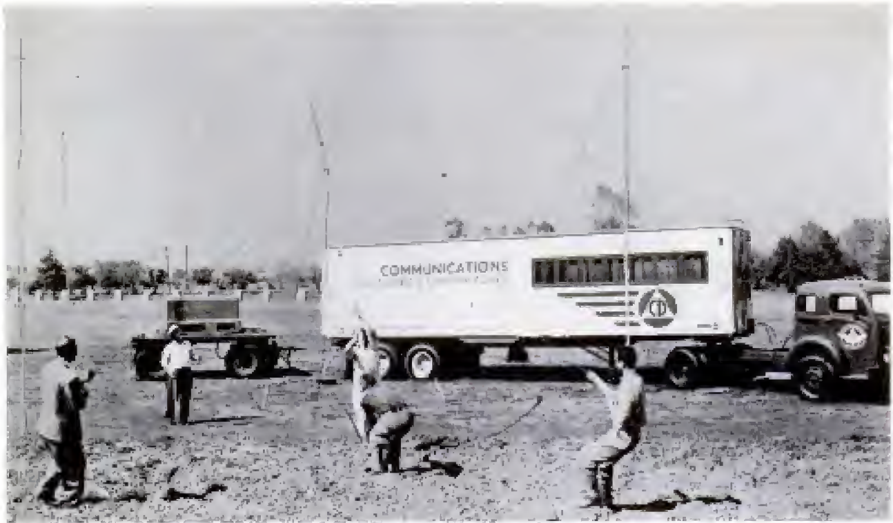
Trailer is towed to safe site and radio antennas erected. Transmitters then relay civil-defense messages
